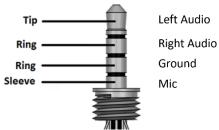
functions can share a single ground connection. With this in mind, look at a typical TRRS connector shown to the right.
