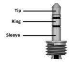
plug has 3 electrically isolated connections corresponding with the tip, single ring, and the sleeve position.
